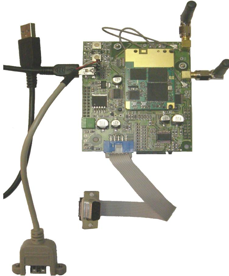
The IoE Gateway board provide local network to remote server gateway features.
